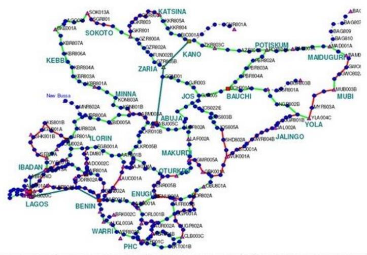
Globacom have a Microwave network that practically spans the whole of Nigeria. On the SDH network the capacity is a minimum STM2 with 1+1 redundancy. This network alongside OFC network is used to carry most of our traffic nationwide.
