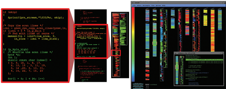
Figure 3.2. Left: SeeSoft representation for software source code where successively smaller fonts lead to a “reduced” single row of pixels per line of source code. Right: Module in a software system with color encoding the age of lines of code.
