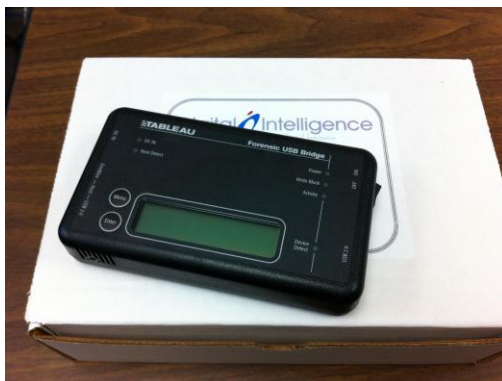
Figure 2: Tableau Forensic Write-Blocker
