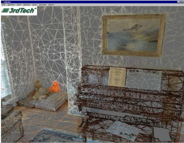
Figure 3. Single 2D picture captured from the same 3D scene capture as figure 2, and seen from the same viewpoint as figure 2, but with the rendering changed to display the polygon with the interior colors turned off. Thus, objects in the picture seem transparent, and the number of polygons used to depict objects can be appreciated.
